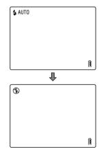
The flash mode icon changes through the cycle shown below each time  $\triangle$  on the 4-way button is pressed.
